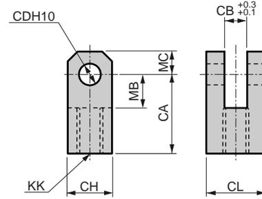
Note: A pin, a washer and a split pin are attached.
