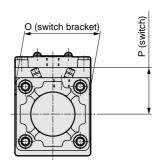
2 color indicator type, preventive maintenance output switch installation dimensions
