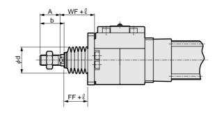
Note 1: Dimensions shown in parentheses are for the rubber cushion type. This type is longer than the air cushion type.
