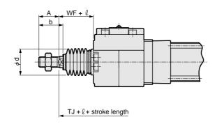
Note 1: Dimensions shown in parentheses are for the rubber cushion type. This type is longer than the air cushion type. ( $\phi$ 40; +6mm,  $\phi$ 50/ $\phi$ 63;+8mm,  $\phi$ 80/ $\phi$ 100; +10mm)
