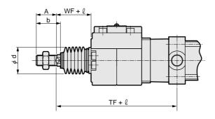
Note 1: Dimensions shown in parentheses are for the rubber cushion type. This type is longer than the air cushion type. ( $\phi$ 40; +6mm,  $\phi$ 50/ $\phi$ 63; +8mm,  $\phi$ 80/ $\phi$ 100; +10mm)
