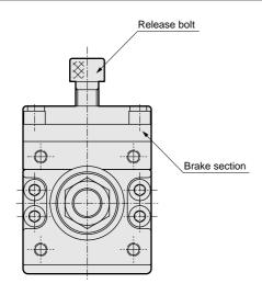
The brakes are released by screwing a bolt into the manual release port (female threads on top of brakes).
