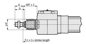
Note 1: Dimensions shown in parentheses are for the rubber cushion type. This type is longer than the air cushion type.  $(\phi 40; +6mm, \phi 50/\phi 63; +8mm, \phi 80/\phi 100; +10mm)$
