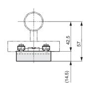
Joint/high load type (RJ-H)
