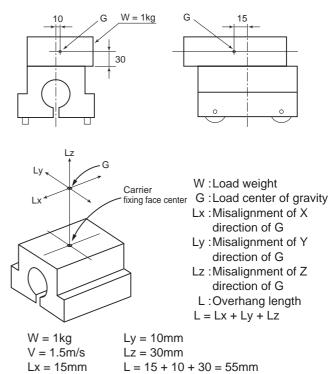
When using with a load weight of 1kg and speed of 1.5m/s, if W = 1kg according to graph (2), the speed is 2m/s and is within the range. However, a deceleration circuit is required.
