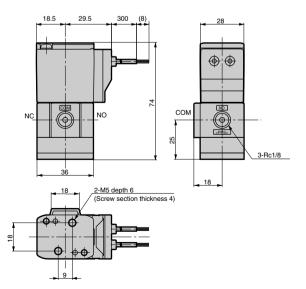
\* When a set screw end in fixing holes 2-M5 is more than 6 mm from the bottom of the mounting plate, the screw cuts into the body or base, leading to cracking. The screw end must be 6 mm or less from the bottom of the mounting plate.
